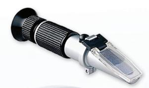
The glycol tester is used to measure the freezing point of either ethylene glycol or proplyene glycol
