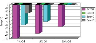
As the graph shows not all ISO 32 POEs are created equal. RPOE LT 32 offers the best low temperature properties available today. When partially miscible lubricants enter the evaporator, the lubricant and refrigerant will separate into two distinct phases, when the temperature falls below the critical solution temperature.
